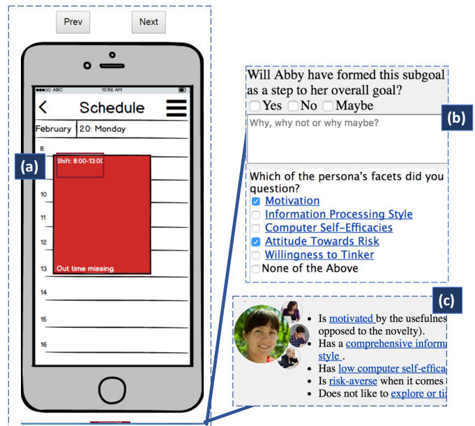
Fig. 1: The Recorder’s Assistant tool during an evaluation of a mobile time-and-scheduling app. (Left): The app being evaluated is displayed with (a) a rectangle around the action the evaluators are deciding if a user like “Abby” will take. (Right): A blow-up of portions of the GenderMag features for the app: (b) the GenderMag question the team is answering at the moment, including a checklist of Abby’s facets; and (c) a summary of the persona the team has decided to use (in this case, Abby).
